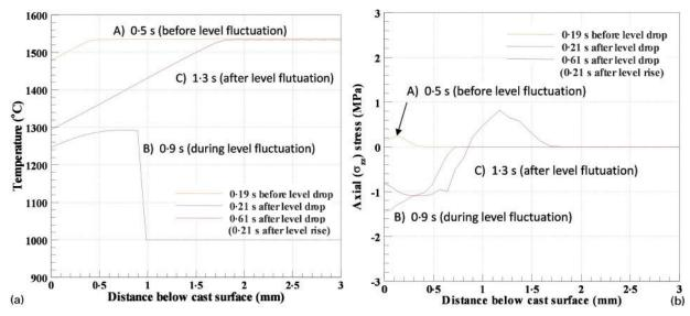
5 Temperature and stress profiles through shell during level fluctuation event (5 mm from bottom edge)
