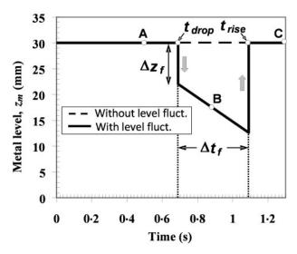
3 Metal surface level history during a simulated level fluctuation in lab (stationary) frame of reference. Instants A, B, and C occur before, during, and after level drop
