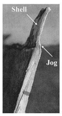
7 Jog shape on inside edge of a breakout shell observed by Fredriksson and Elsber<sup>10</sup>
