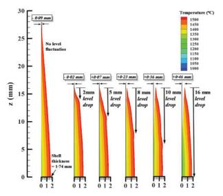
6 Effect of level drop distance on shell temperature and distortion (ULC steel)
