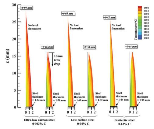
8 Simulated shell distortion for three steel grades with and without level fluctuations: the ULC and peritectic steels exhibit more thermal distortion (compositions given in Table 1)
